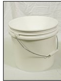
Buckets For mixing grout in and for clean water.
